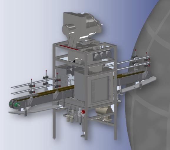
Simple, cost effective on-line ultrasonic spray coating to dramatically reduce container static & external scuffing & improve bottle handling
