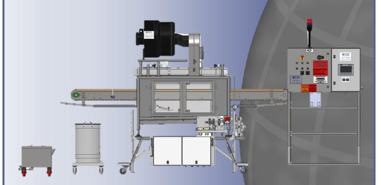
Simple, cost effective on-line ultrasonic spray coating to dramatically reduce container static & external scuffing & improve bottle handling
