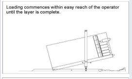
The pallet is lowered by pressing the foot pedal leaving sufficient space for the next layer. The loading cycle continues until the pallet load is complete.
